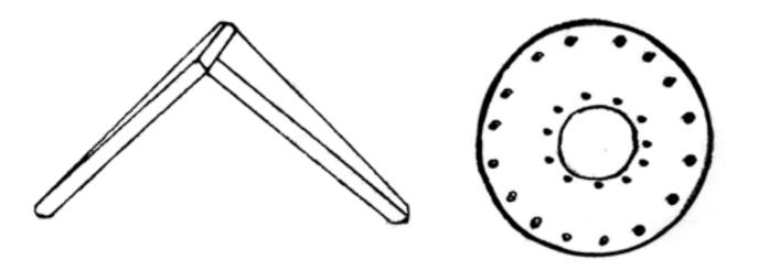
A **lens shield**, shown on the left, is attached above the lens hole. On the right is a **compact disc** with nails on the inner and outer rim; this is fitted over the lens hole.
